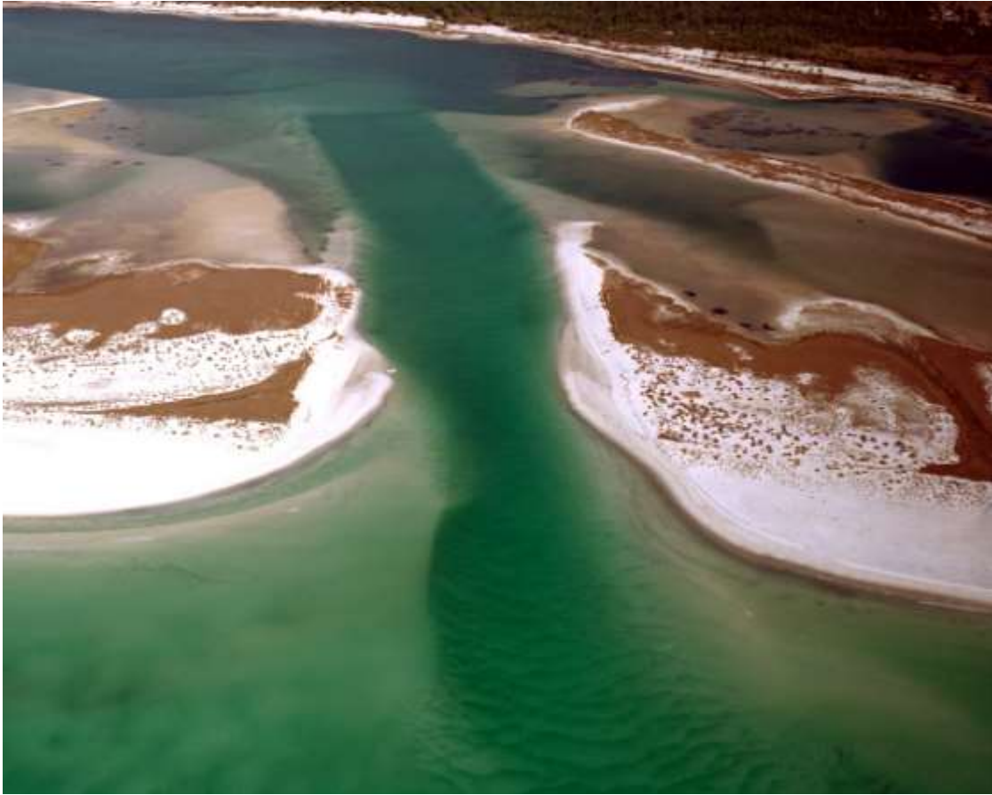
Photo 1. Aerial photo of the East Pass Experimental Re-opening following construction in December 2001.
